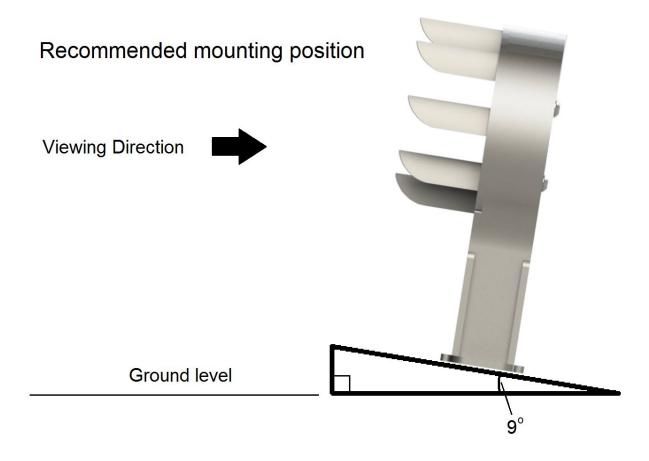
For best viewing at close distances mount the CPL at aproxamately 9 degrees. This gives the best view at ten (10) feet distance. A 9 degree angle is 1 inch rise over 6 inches run. The picture above depicts a true 9 degree angle for reference.
