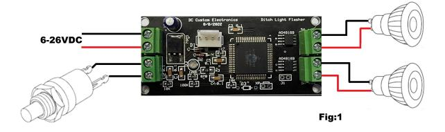
\*\* Note: Trigger is Sink only. This means to trigger, the input must be connected to 0V or "ground" To wire this with a horn see Figure 2
