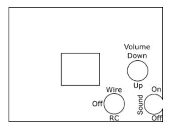
To power on the control box for RC (remote control) mode, put the power switch in the "RC" position.
